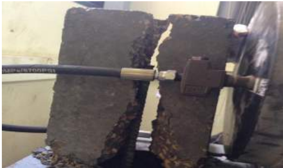
Fig 4.15: Samples in Bonding test at second phase.
