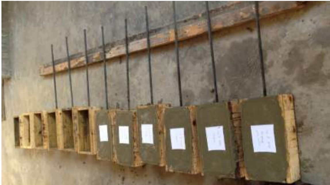
Fig 4.2: Corrosion process in the first phase of test program.
