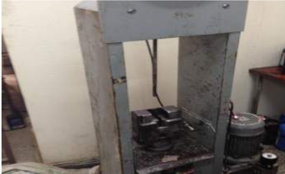
Figure 3.11 Pull out test machine
