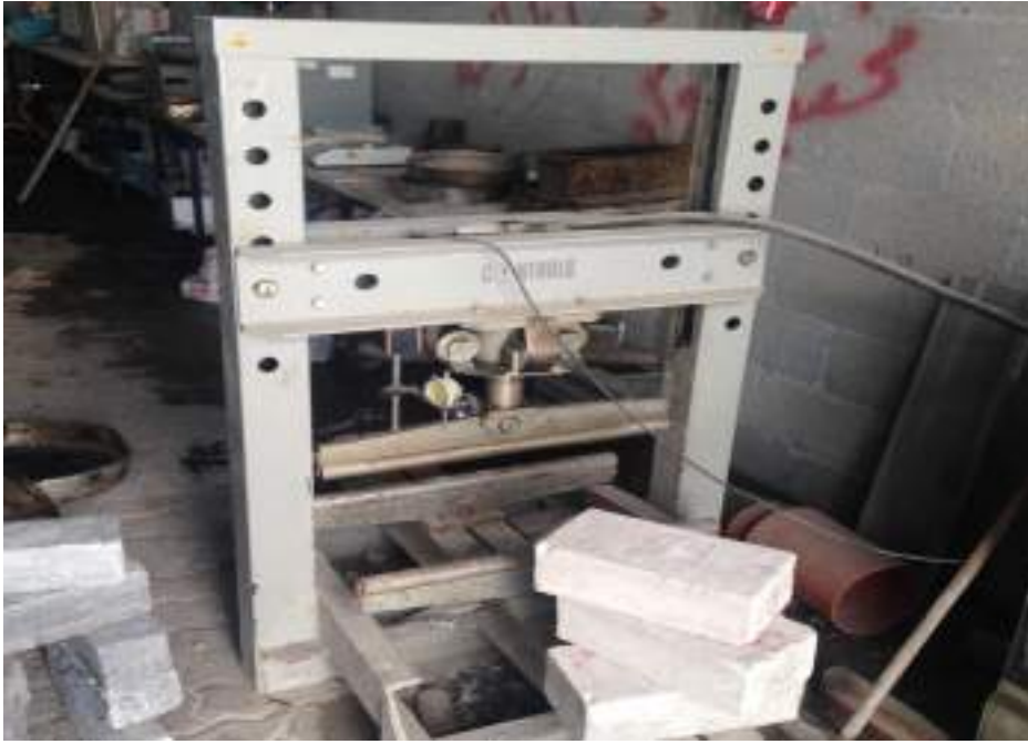
Fig 4.17: Flexural Tests in the second phase of test program.
