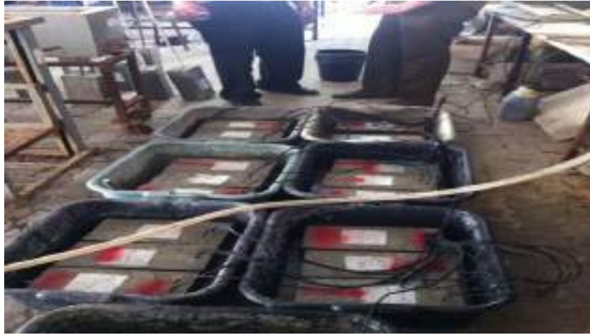
Figure 3.10 Connection of samples with electrical cell
