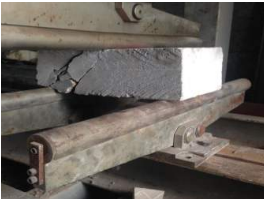
Fig 4.18: Flexural Tests in the second phase of test program.
