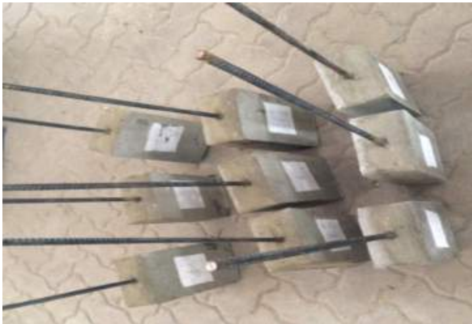
Fig 4.12: Samples in Pull out Force test.
