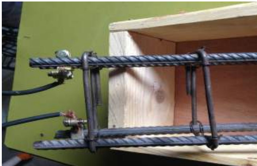
Figure 3.9 Connection of reinforcement with electrical cell
