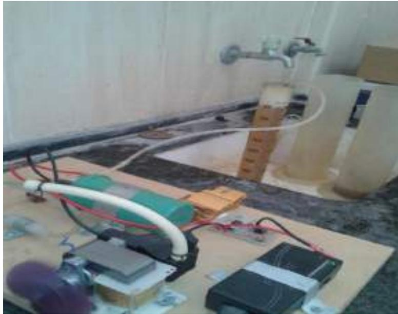
Figure (3-4) disinfection by ozone for the first sample 0.5 liter
