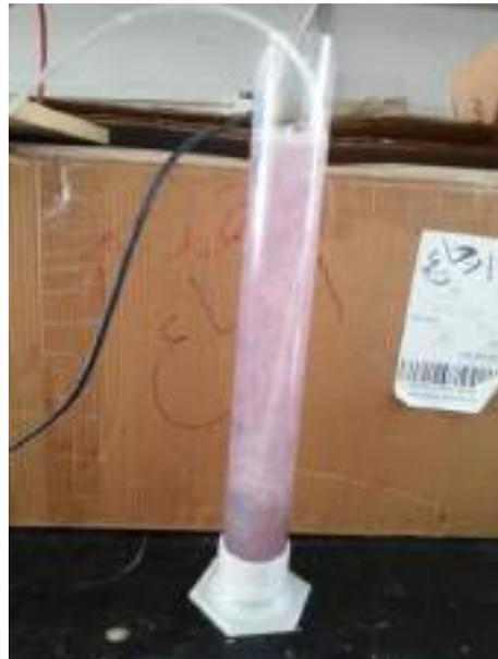
Figure ( 3-3 ) : pump ozone in the sample to calculate ozone concentration
