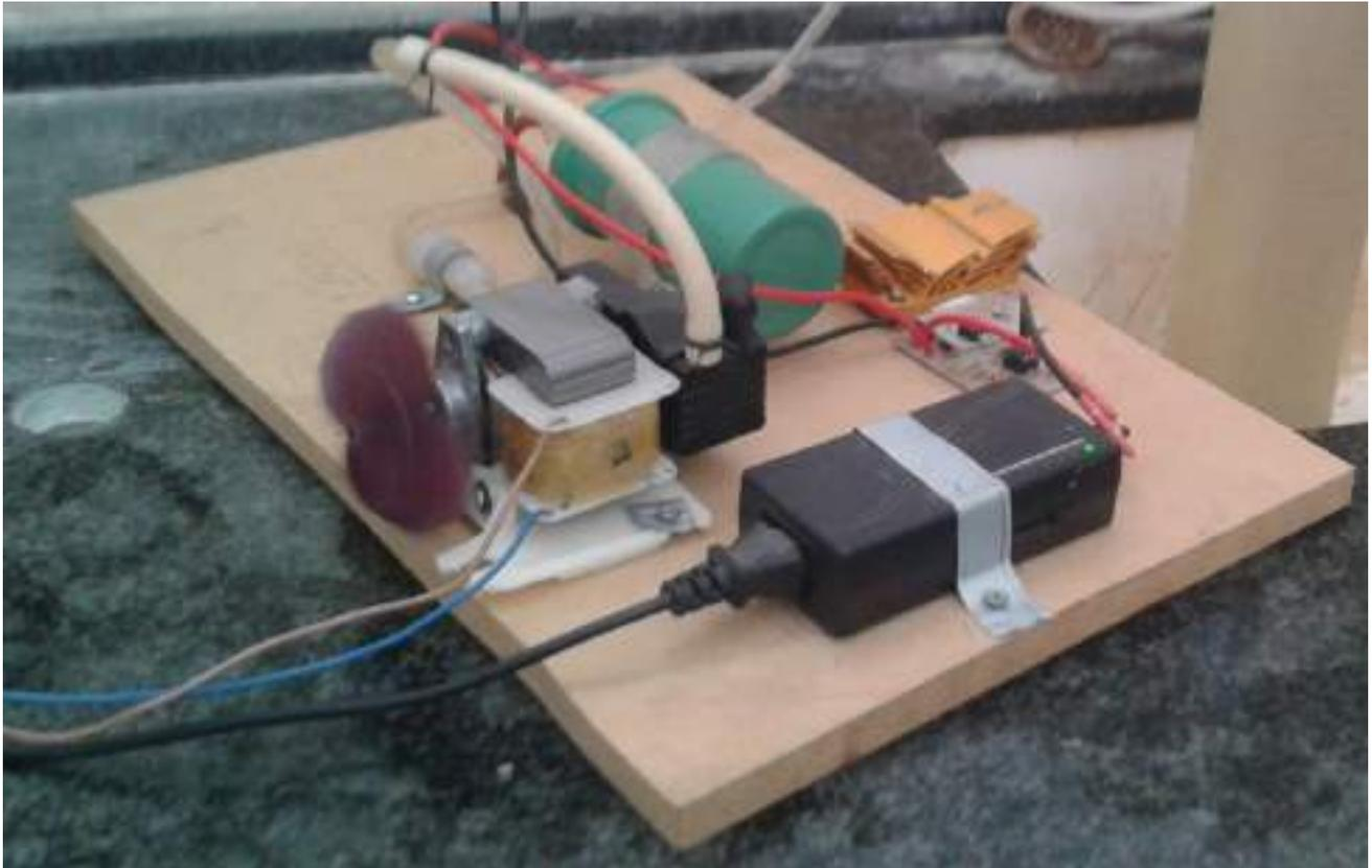
Figure ( 3-2) : ozone generator device with all component
