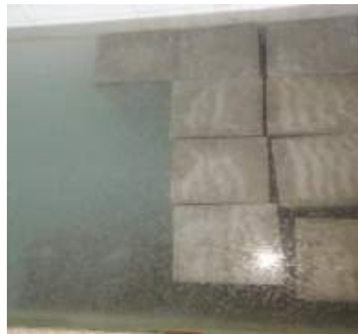
Figure 3.11 : Cubes at curing basin
