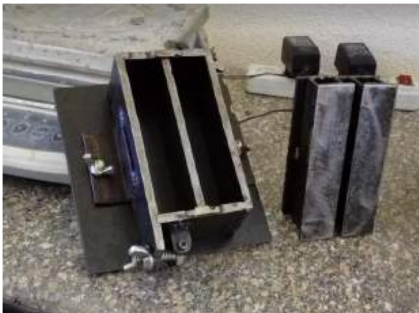
Figure (4.2): Steel molds used in preparing asphalt beams
