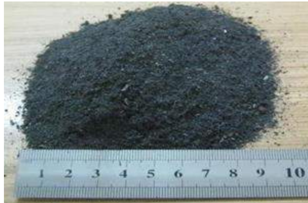
Figure (3.6): Used gradation of Iron powder (0 – 0.60mm)
