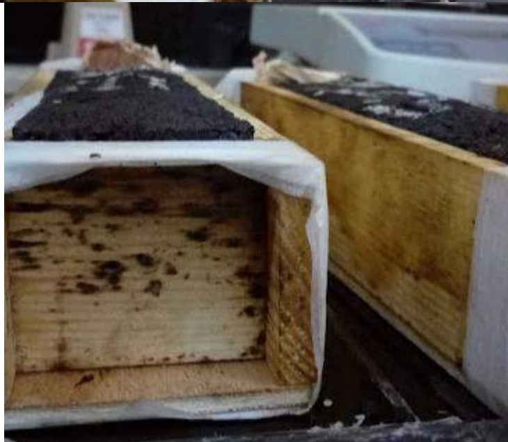
Figure (5.16): Visually observed deformities for sample surface with 10.0% iron content, after getting heated above 170 °C
