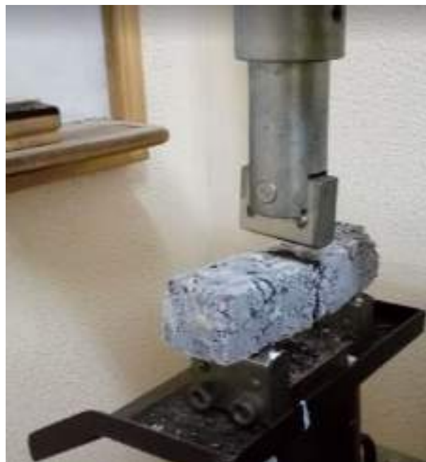
Figure (4.4): Using three-point bending in testing samples
