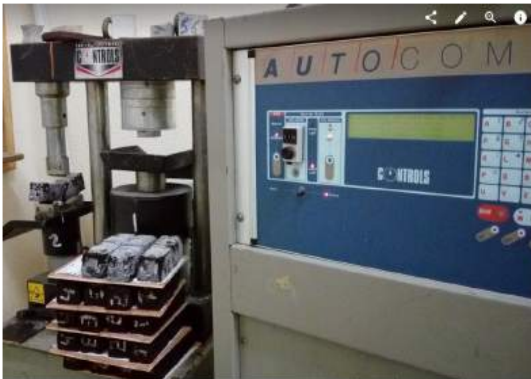
Figure (5.12): Using three-point bending testing machine to measure fracture point load
