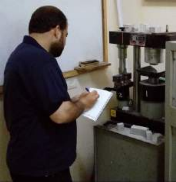
Figure (F7): Samples fracture with three point bending machine
