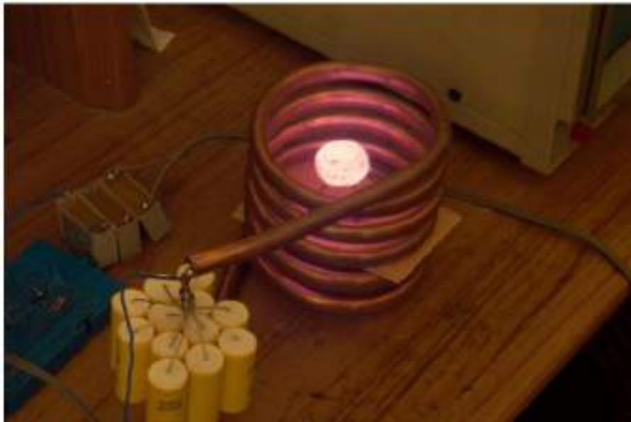
Figure (2.3): Steel nut heated by induction heating coil
