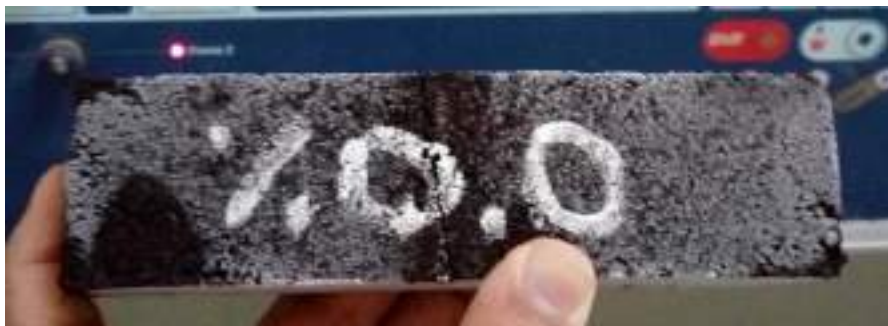
Non-Cracked sample (0.0% Iron Content)
