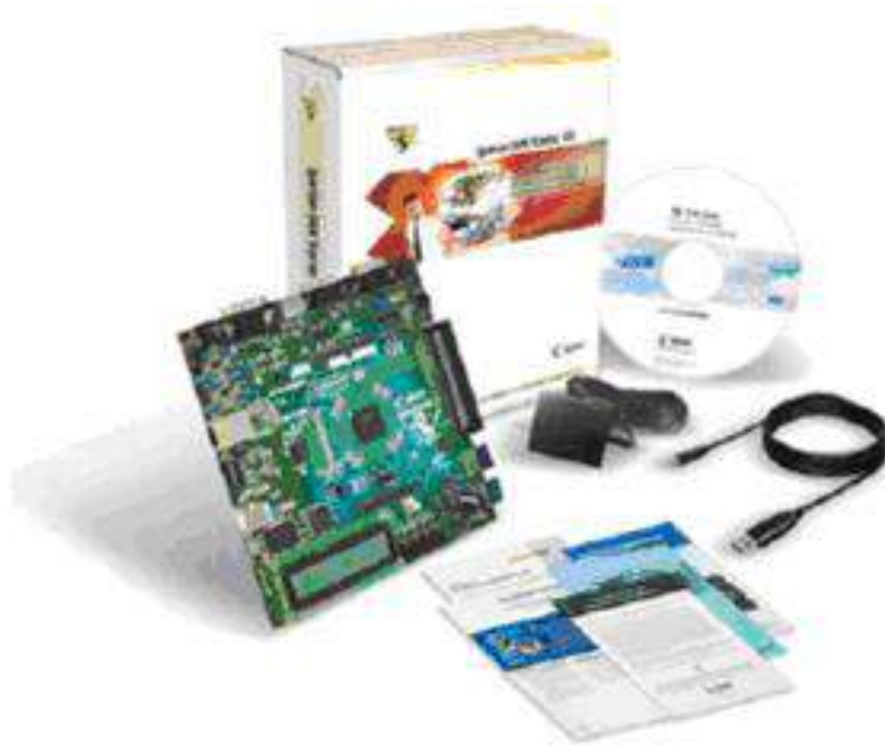
Figure 4-11: Spartan-3AN Starter Kit Board .
