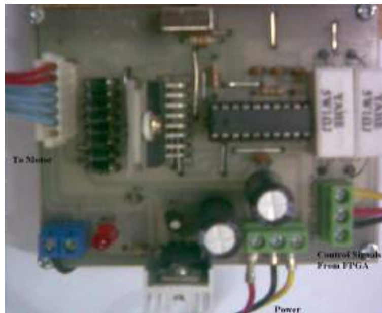
Figure 5-22: Stepper motor driver PCB kit.
