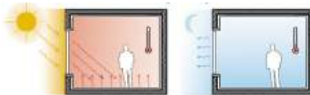
Figure (4.9): The effect of thermal mass of heavy building materials during day and night, (Mikler et al., 2008)
