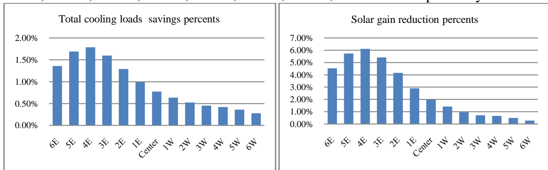
Figure (4.42): Energy savings percents in summer and solar gain reduction percents (in south façade)
