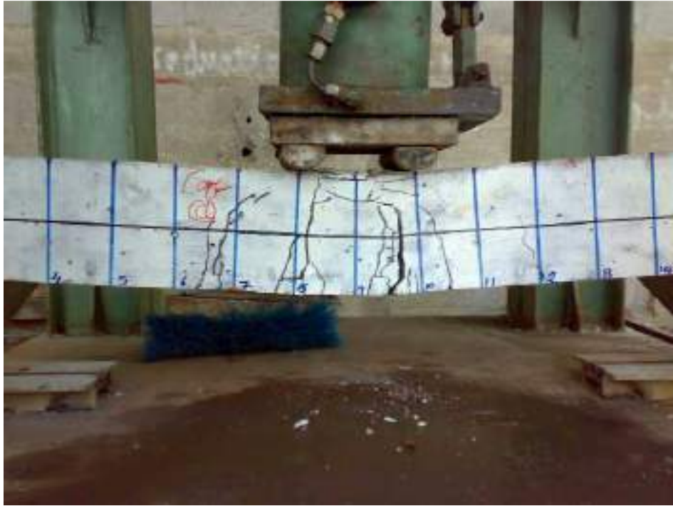
Figure 5.19: Crack Pattern Photo for Beam (Co.B1) At Failure
