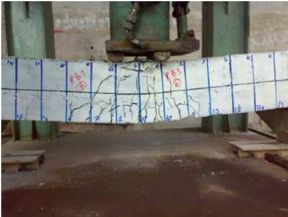
Figure 5.22: Crack Pattern Photo for Beam (R3-B2) At Failure
