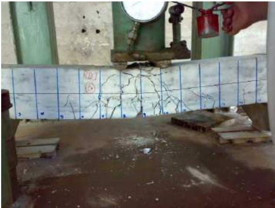
Figure 5.20: Crack Pattern Photo for Beam (R1-B1) At Failure
