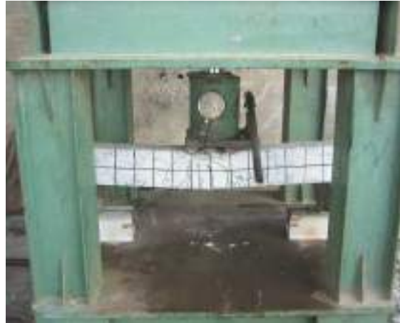
Figure 4.5: flexural test machine (I.U.G. Laborite's Machine)
