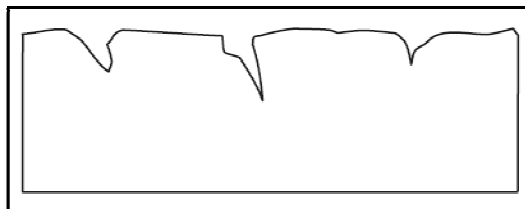
Figure 2.6: Pitting Corrosion (El-Reedy, 2008)
