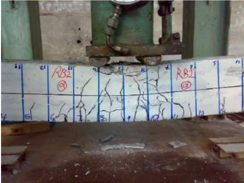
Figure 5.21: Crack Pattern Photo for Beam (R2-B1) At Failure
