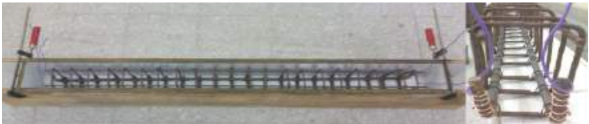
Figure 4.8: Wood Form and Reinforcement Details
