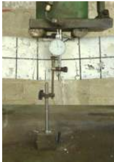
Figure 4.16: Deflection Dial Gage Fixation
