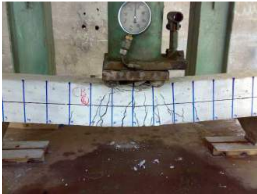
Figure 5.18: Crack Pattern Photo for Beam (CB2) At Failure
