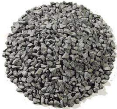
Figure 4.12 Coarse aggregate (crushed basalt) ranges from 2-9 mm.
