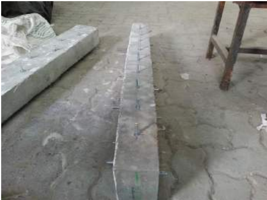
Figure 3.3 Distribution of (HSA M8 35/25/-) Hilti type anchors.
