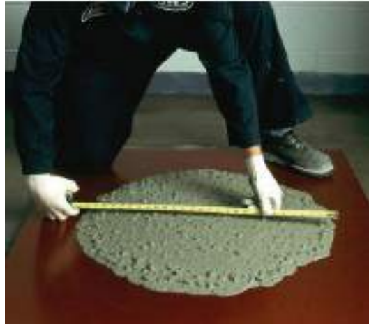
Figure 4.11 Self-Compacting Concrete. (Source: Technical Bulletin, 2005, P1)
