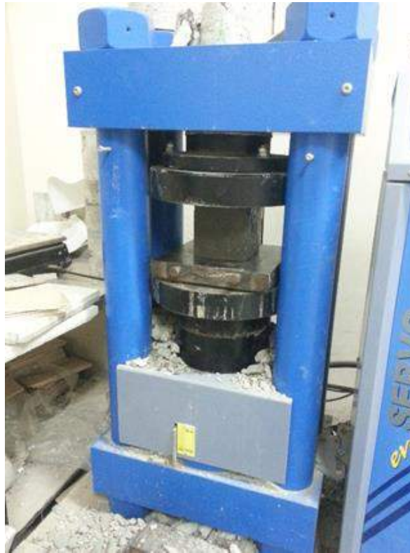
Figure 4.4 IUG Lab compressive strength test machine.
