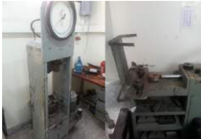
Figure 4.5 IUG lab. standards tensile strength test machine.
