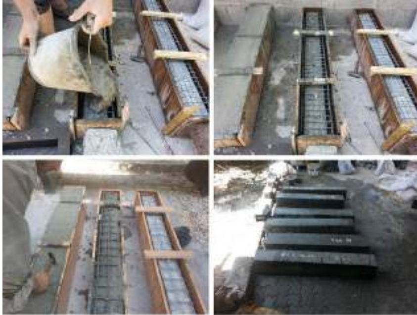
Figure 4.24 SCC casting process.
