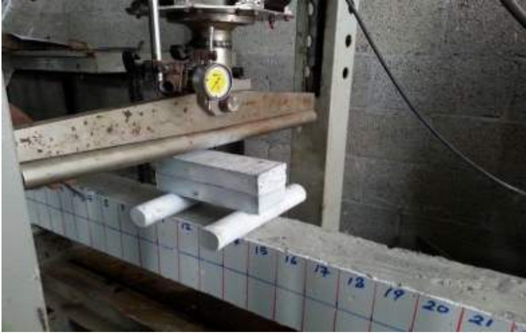
Figure 4.26 Flexural machine at IUG and deflection dial gauge fixation.
