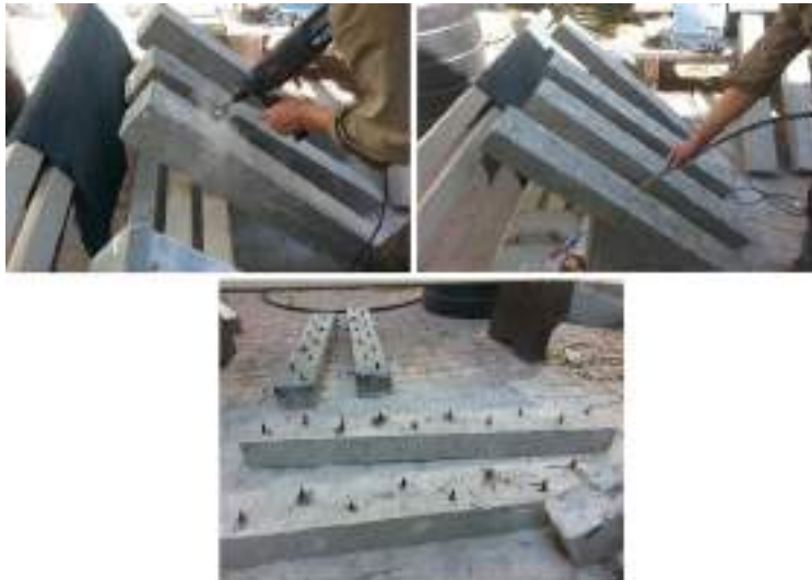
Figure 4.21 Shear connector distribution.
