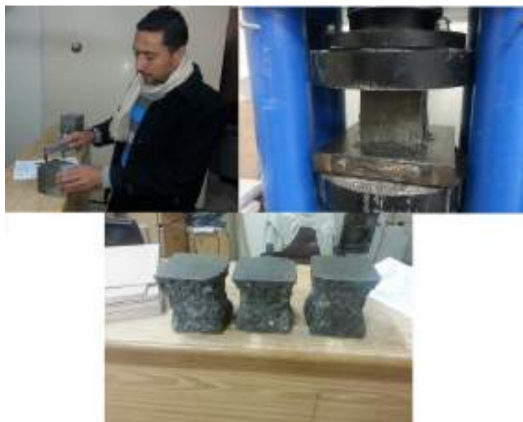
Figure 4.17 SCC compressive strength test.
