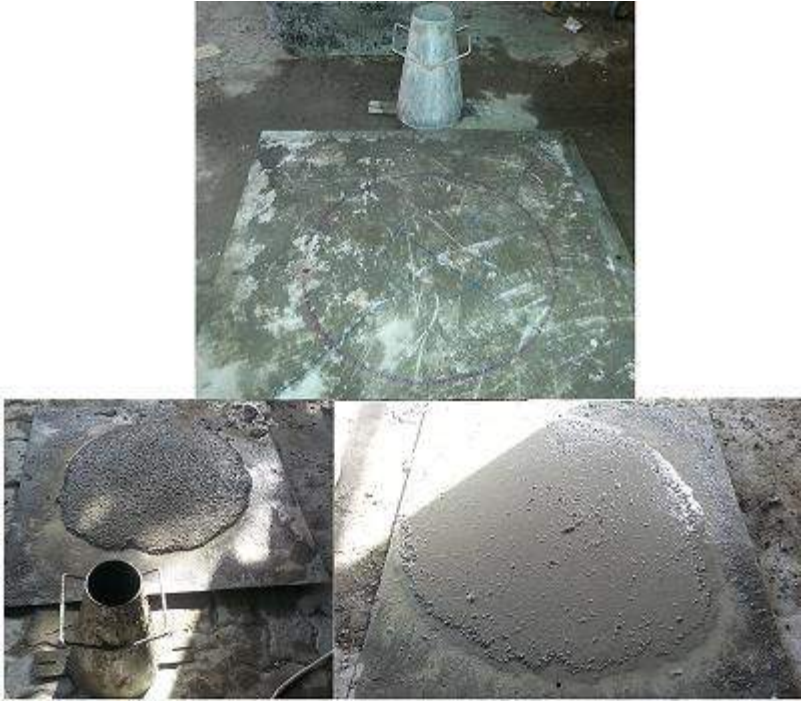
Figure 4.14 T500 and slump flow test.
