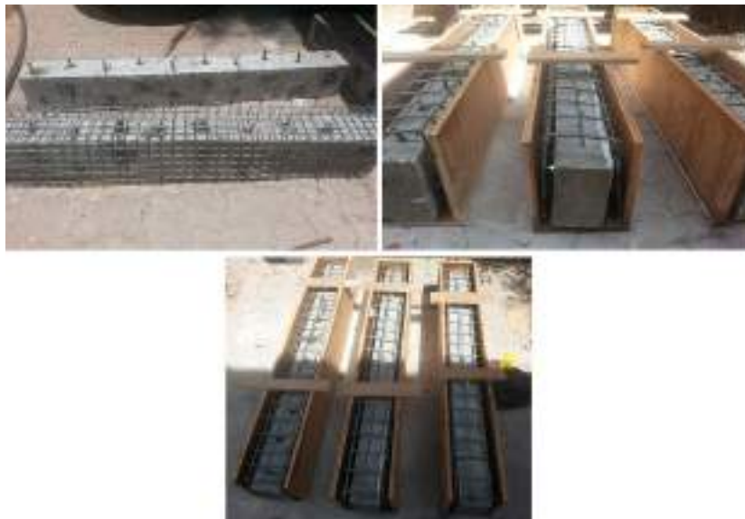
Figure 4.23 Wooden molds with specimen preparation.
