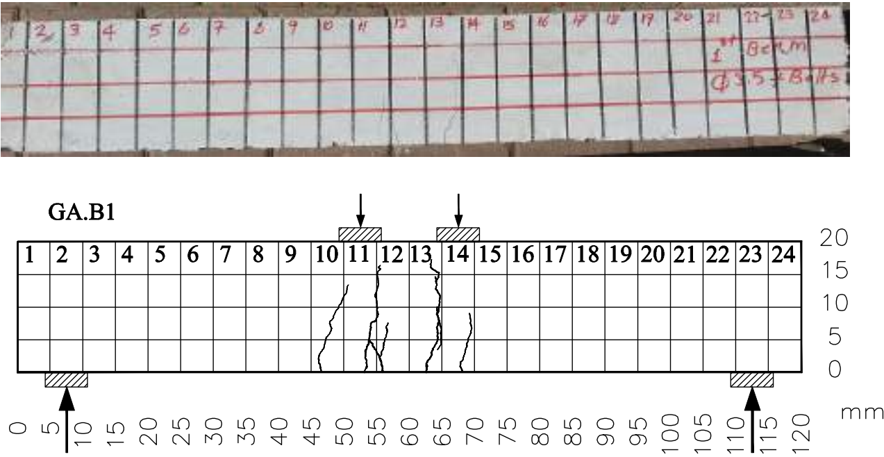
Figure 5.11 Failure mode and crack pattern of GA.B1.
