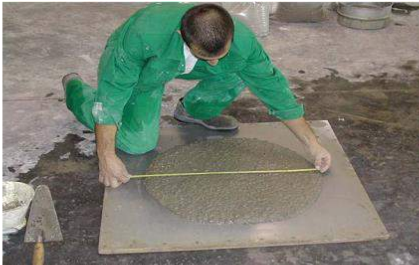
Figure C.2 SCC flow spread measurement. (Source: EFNARC, 2005)
