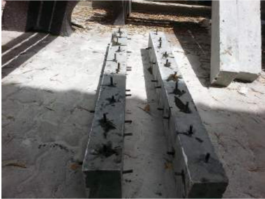
Figure 3.2 Distribution of 8 mm steel deformed bar anchors.
