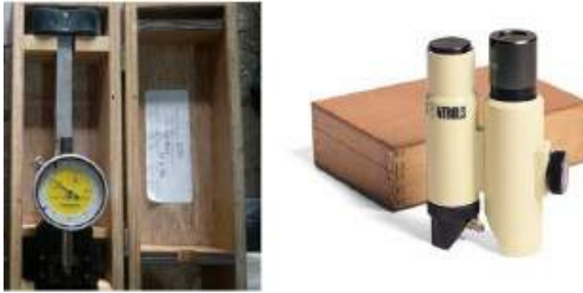
Figure 4.27 IUG's displacement gauge and microscope meter.
