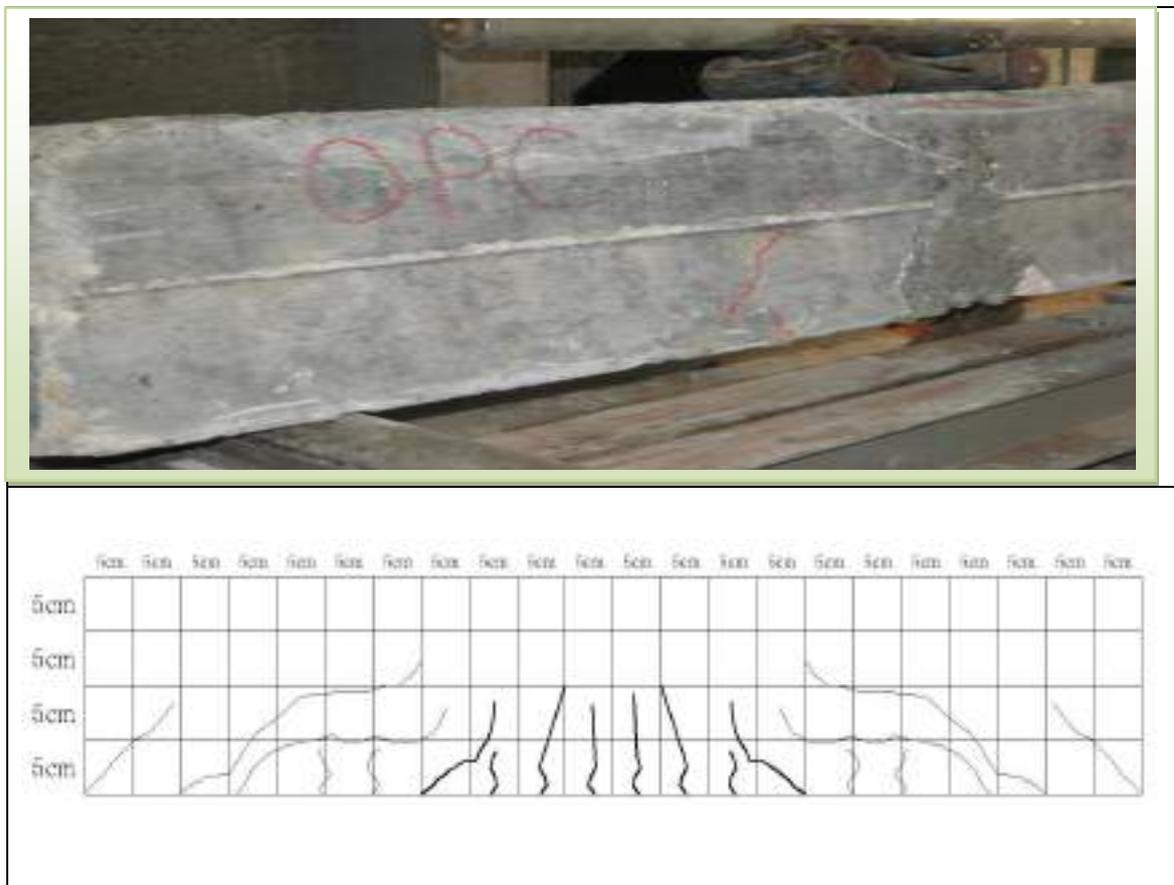
Figure 5-14: Honeycomb beam repaired by OPC tested, and its crack pattern
