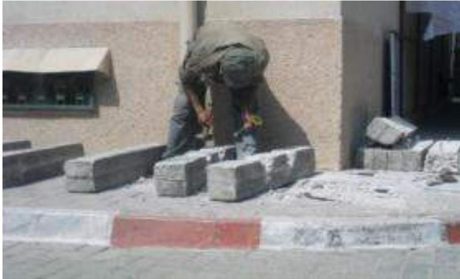
**Figure 6-5: chip the concrete cover of the heated samples**
