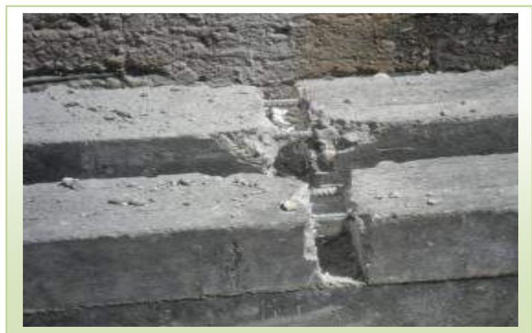
**Figure 5-4: Cleaning the honeycomb samples**
