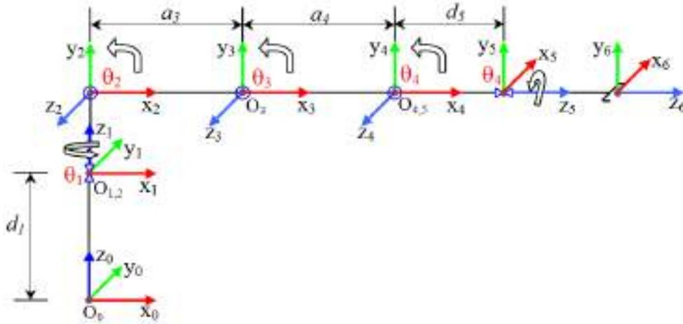
**Figure (3.2): Coordinate Frames of AL5B Robotic Arm**
