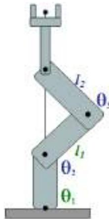
**Figure (4.2): Internal Singularities Type**
