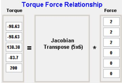
Figure (7.19): Example 4 Torque - Force Relationship
