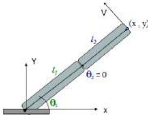
**Figure (4.1): 2-DOF planar manipulator fully stretched out**
