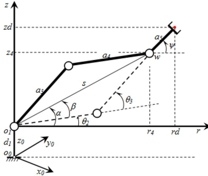
Figure (3.4): Planar View of AL5B Robot Arm.
