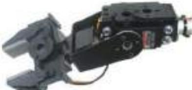
**Figure (A.6) Wrist and gripper**
