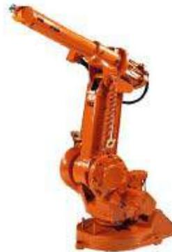
**Figure (2.3): The ABB IRB1400 Robot.**
