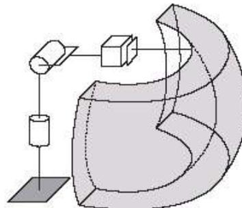
**Figure (2.9): Workspace of the Spherical Manipulator.**
