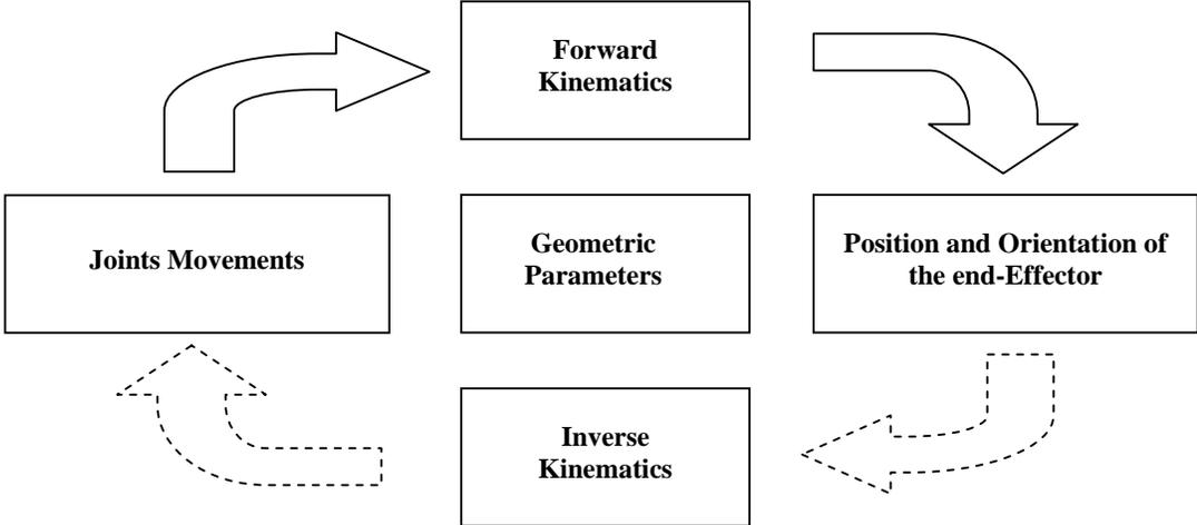
Figure (2.20): Kinematics Block Diagram
