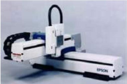
Figure (2.17): The Epson Cartesian Robot.
