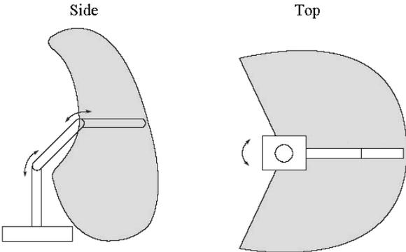
Figure (2.6): Workspace of the Elbow Manipulator.
