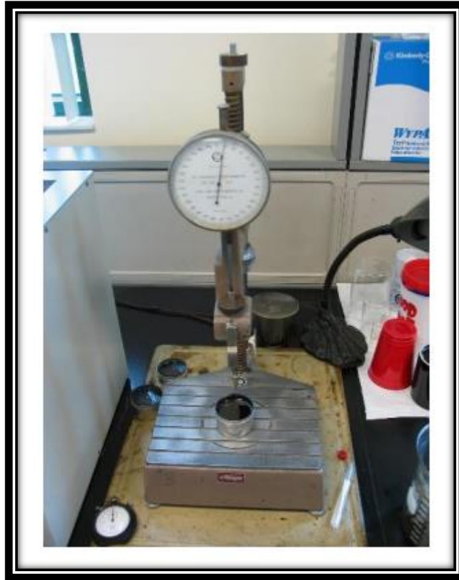
Figure 3.2: Penetration test for a bitumen sample bitumen properties
