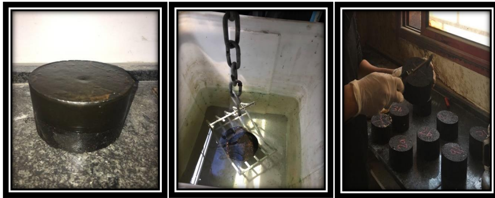
Figure 4.18: Bulk density testing of MA specimens.
