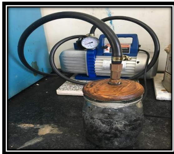
Figure 2.4: specimen in Gmm testing device
