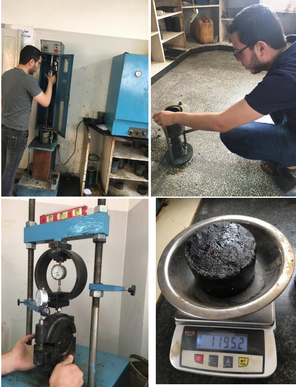
Figure 5D.1: Preparing mixtures and testing Marshall stability & flow
